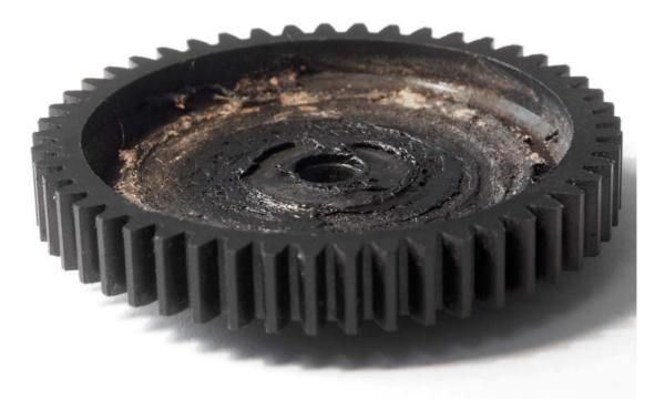
This picture shows, where the spur gear melts if the slipper clutch is set too loose. The slipper clutch is only meant to slip under extreme loads and is on the car to save the transmission from serious damage.
