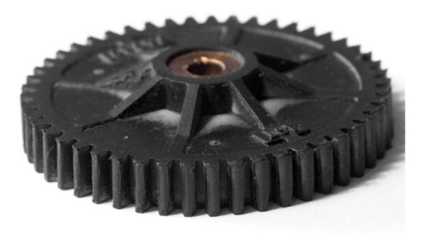
If the clutch bell gear and the spur gear are not meshed correctly then the spur gear can be damaged as shown in the picture above.
