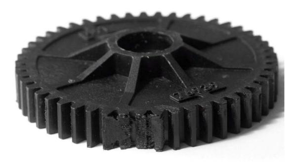
This picture shows the damaged caused by a hot clutch bell. Only a few teeth have melted.
